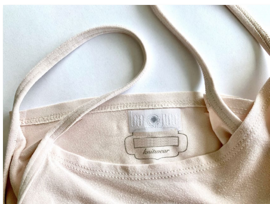
Datamars Laundrychip 403 heat-sealed on a personal garment
