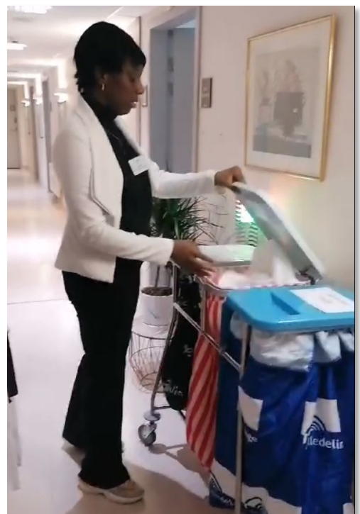
The “Sorti-Cart” in action: when a personal garment is thrown into the wrong bin, the red-light-buzzer alerts the operator.
