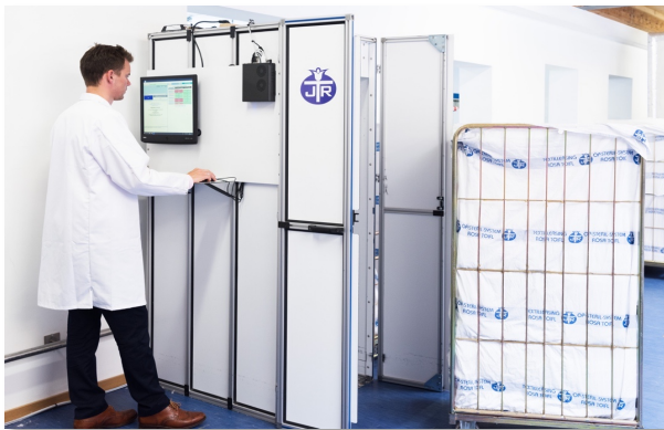
Picture 4: RFID reading cabin for bulk detection of entrances and exits.
