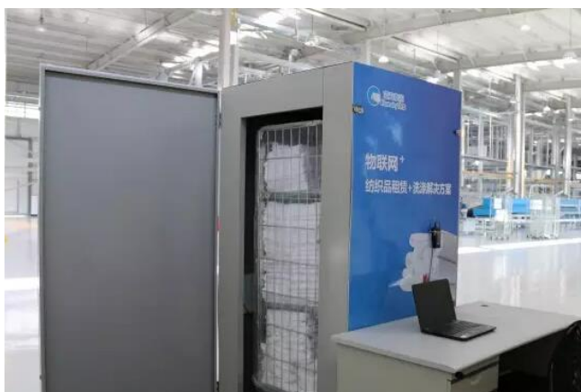
Fig. 2 – Trolley with clean textiles read by the RFID cabinet.
