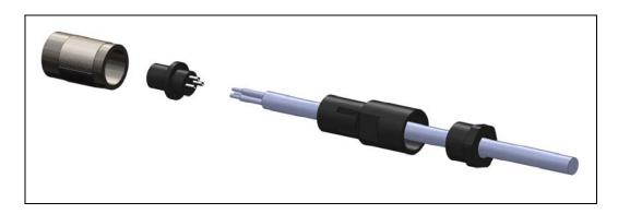
The 3 wire terminals must be soldered on the connector terminals as described in chapter 1.1.
