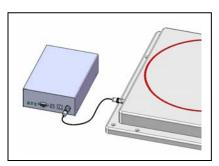
2. Connect the serial white cable from the connector marked "Host" to any serial port (COM) on your PC or the reader "R-IN 1300 MID" can be connected to the LAN just like a PC (Ethernet cable & RJ-45 connectors).
