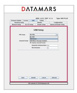
Select from the "USB usage" options the desired functionality (serial disabled, serial emulation, mass-storage emulation).
