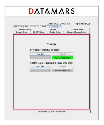
The average value is computed and shown in the box below the Stop SNR button.
