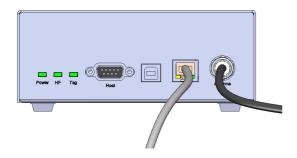
A direct Ethernet connection between a PC and "R-IN 1300 MID" reader is also possible, with an *Ethernet Cross Cable* (supplied together with the reader). Refer to Appendix A for more details on how to do this.
