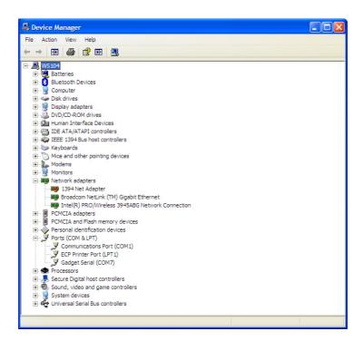
**NB:** If the USB-Cable is unplugged, the USB-Serial-Communication stops. If now you plug the USB-Cable in, the USB-Serial-Communication will NOT start! After unplugging, you have to close the terminal, plug the USB-Cable again and open a new terminal.
