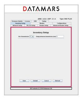
The "InventoryrSetup" tab allows users to specify into more details how the TableTop-Antenna works in a non-continuous mode set-up.
