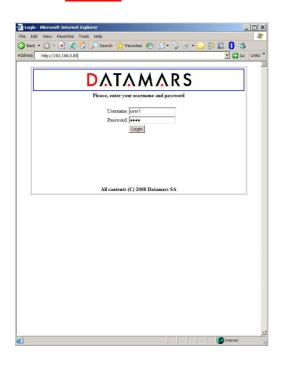
The interface running on the browser permits access to users only via login (user name & password): attempts to join the configuration- and monitoring tools directly via bookmarks are prevented from the system.
