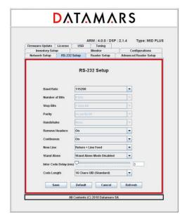
The "RS-232 Setup" allows users to specify the properties of the serial connection.
