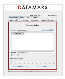
The GUI-version running on the browser offers the user a tool to update the software of the "R-IN 1300 Reader".
