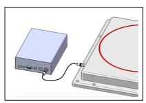
You can not use cable other than the 3.5m coaxial 50Ω cable supplied by Datamars. Additional extension cables at disposal.
