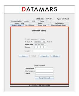
The "Network Setup" tab allows users to specify network parameters: IP address, sub-mask and default gateway. The IP address can be a fixed IP-Address (in this case the ip-address and port must be specified) or a dynamic one (DHCP) [not yet available]. After having changed any network parameters, the browser must be closed and a new login must be done using the new network setup of the reader.
