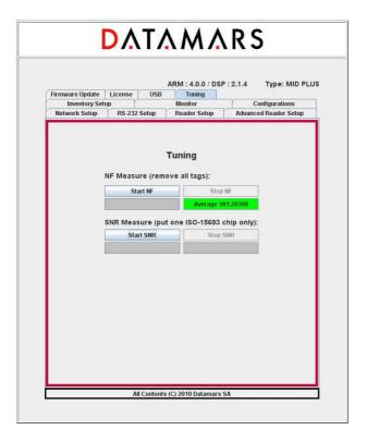
To stop the NF measurement, press the STOP NF button. The average value is computed and depicted in the coloured box.
