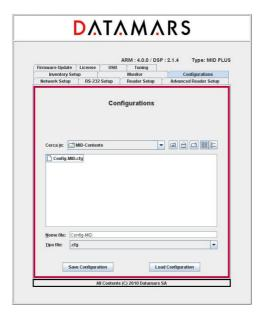
The "R-IN 1300 Reader" offers a tool giving the user the possibility to save and/or reload configuration files.
