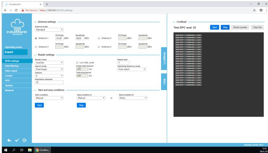
Cloudburst allows to set-up all the parameters included the network interface of the reader to connect it to the laundry network and start getting EPCs in the laundry management software.
