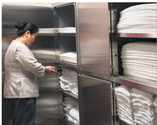
Linen inventory check performed with a handheld RFID reader powered by Impinj E Family Reader ICs with support for Gen2X.
