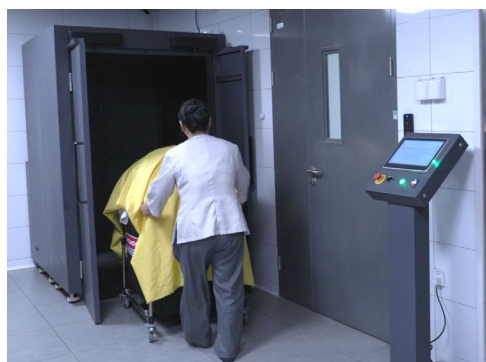
Soil linen outbound scanning performed through a high-density RFID cabinet
