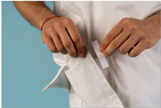
Prototypes of workwear with RFID Laundrychip. Photo: © HSLU CC P&T (2025)
